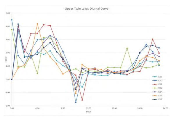
Figure 4. Hourly peaking factors for the Upper Twin Lakes Subsystem
