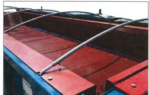
Bolt-in liners are easily removed.
