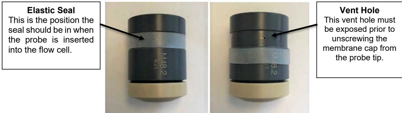
Figure 4: Elastic Seal and Vent Hole on the Chlorine Sensor
