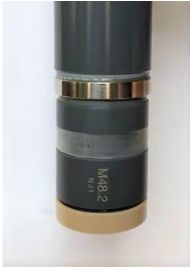
Figure 8: Elastic Seal Covering the Vent on the Membrane Cap
