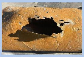
recent years, the District has experienced an increasing number of pipeline failures due primarily to corrosion and material degradation.
