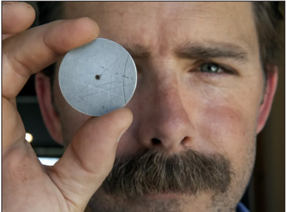
Cason Gilmer, Field Customer Service Representative for LVMWD, peaks through the 1/16-inch hole of a flow restrictor (photo courtesy Mel Melcon / Los Angeles Times)
