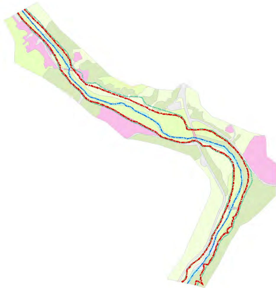
Figure 4.4 – Delineation of Study Area by Varying Roughness Coefficients
