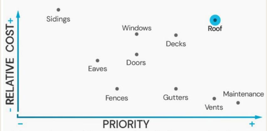
**Relative cost:** Indicates the relative cost of upgrading the listed features to ember-resistant materials and design.
