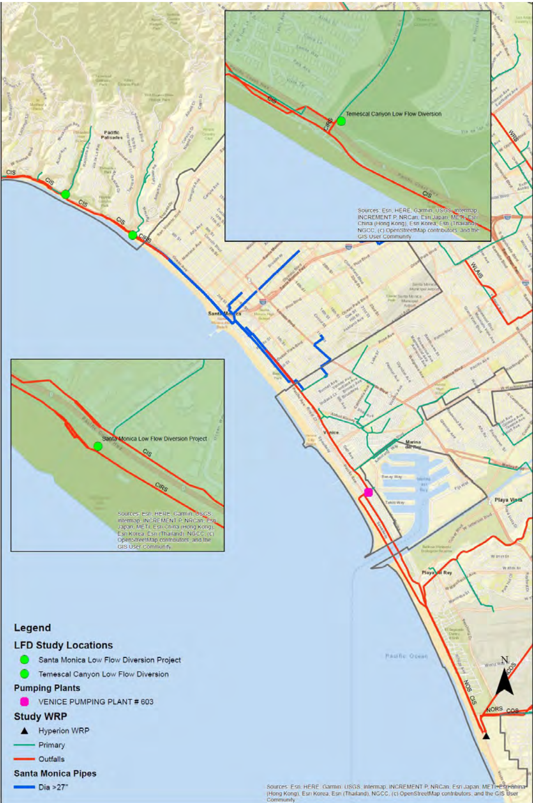
Figure 4-23. Sanitary Sewer System between the Temescal Canyon DWD/Santa Monica Canyon DWD and the Hyperion WRP through the VPP
