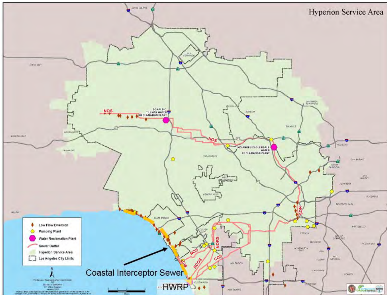
Figure 4-21. Conveyance System – The Hyperion WRP Service Area and the Sanitary Sewer System from Santa Monica Canyon to the Hyperion WRP
