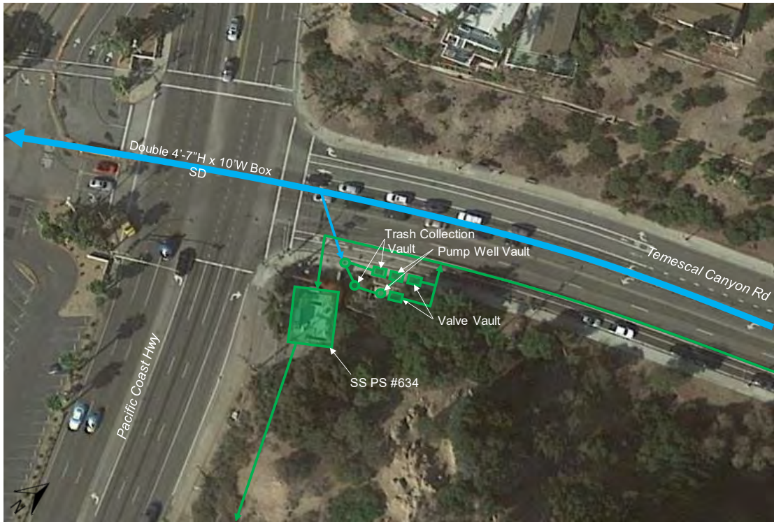
Figure 4-26. Temescal Canyon DWD Location and System Components
