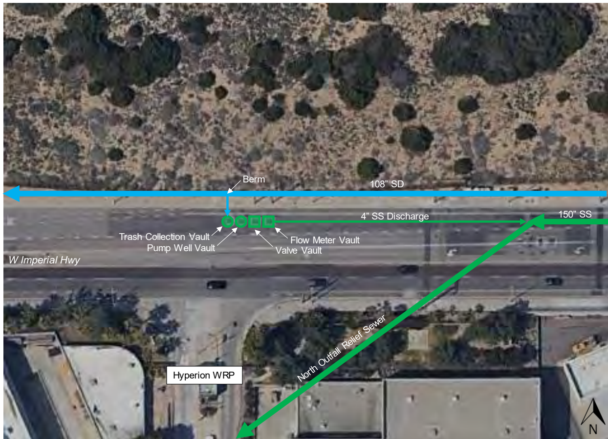
Figure 4-37. Location of the Pershing Drive Dry Weather Diversion Discharging to the Hyperion WRP
