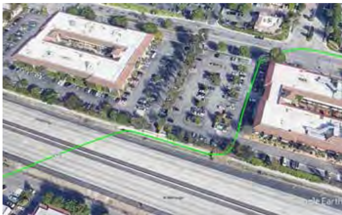
Alignment of the Storm Drain and Caltrans Channel (section running parallel to Hwy 101) accommodating Discharge Point 005. LVMWD has a compliance schedule to address the Discharge Point 005 chloride limitation to the LA River; identifying alternative emergency discharge strategies could be part of the LA River chloride compliance plan.
